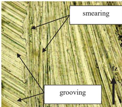
Figure 2 Smearing and grooving occur along cutter locus those effects on Ra reading (20 x).
