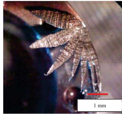
Figure 3 Incomplete segmented anise-like chips appearing during machining, indicating the end of tool life.
