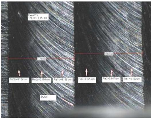
Figure 1 SEM Micrograph of roughness that vary at different locations of cutting path.
