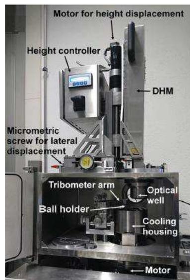
Figure 1 Picture of the high temperature, high vacuum tribometer, combined with a digital holographic microscopy (DHM).
