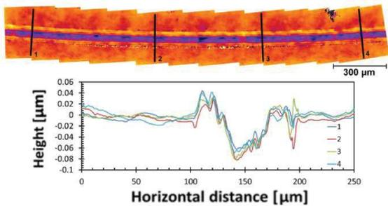
Figure 4 Panorama view of the wear track on a length of 2.5 mm taken by DHM and four selected profiles.
