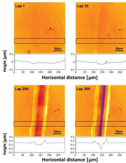
Figure 2 Evolution of wear track at a fix location for various numbers of laps (1, 10, 200, 300 laps).
