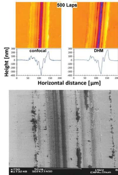
Figure 5 Sample wear images at 500 laps with DHM (top right), confocal (top left) and SEM techniques (bottom) showed that DHM is in good correlation with other imaging techniques.
