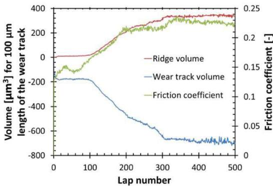
Figure 3 Friction coefficient, ridge volume and wear track volume versus lap number.
