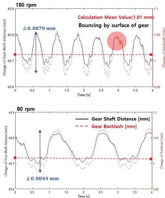
Figure 3 The test results of gear coated silver film.
