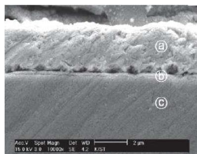
Figure 1 SEM analysis on the silver coating substrate.
