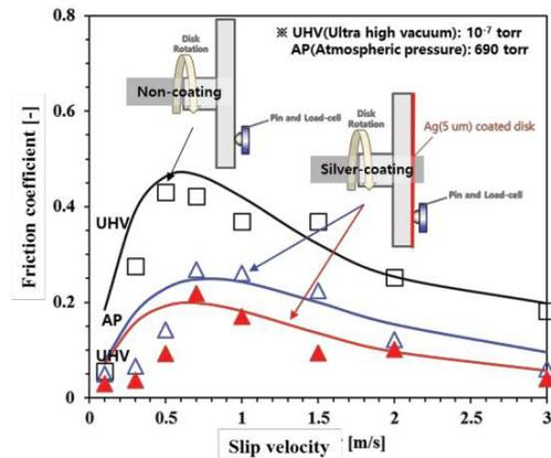
Figure 4 Friction results under the high vacuum.
