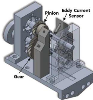
Figure 2 Space Tribo-component Test rig.
