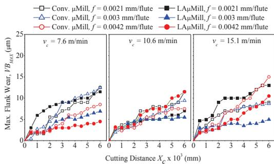
Figure 2 Comparison on maximum flank wear ( $VB_{MAX}$ ) propagation between different feed ( $f$ ) and machining method at  $t_c$  of 0.02 mm.
