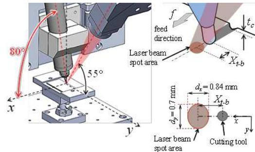
Figure 1 Laser assisted micro milling.
