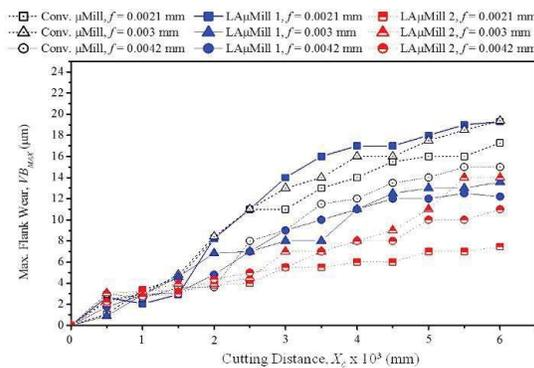
Figure 3 Flank wear increment comparison between Conv.  $\mu$ Mill, LA $\mu$ Mill 1 and LA $\mu$ Mill 2.
