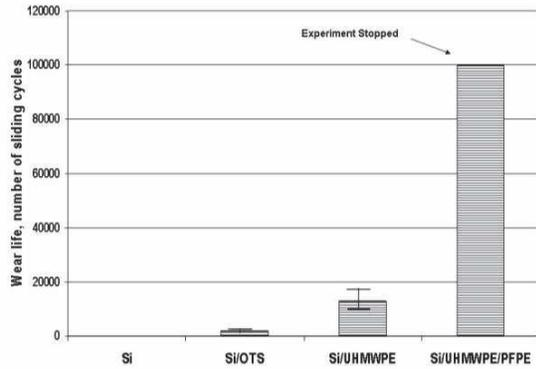
Figure 1 Wear life as the number of cycles of sliding before the coefficient of friction reach the level of 0.3 of bare Si, Si/UHMWPE and Si/UHMWPE/PFPE samples.
