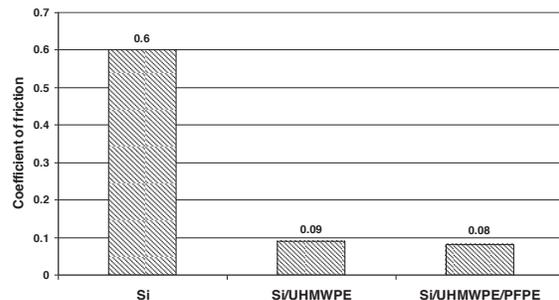
Figure 1 Coefficient of friction of bare Si, Si/UHMWPE and Si/UHMWPE/PFPE samples. Tests were conducted at 70 mN load with calculated contact stress of 370 MPa and sliding speed of 0.042 m/s and the counterface was a 4 mm diameter silicon nitride ball [1].
