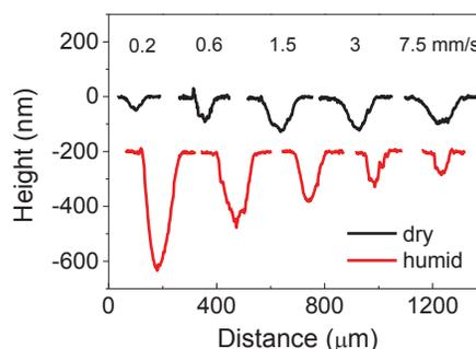
Figure 1 Profile lines of wear tracks in phosphate glass under various sliding velocities in dry and humid air.
