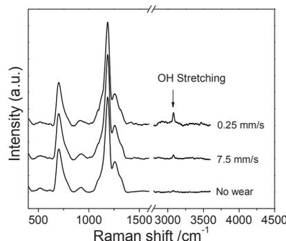
Figure 3 Raman spectra of the wear debris in phosphate laser glass after wear testing in humid air.
