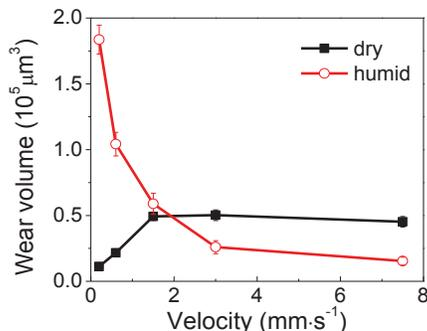
Figure 2 The wear volume of phosphate laser glass as a function of sliding velocity in dry and humid air.
