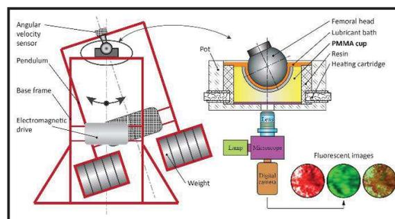
Figure 1 Schematic illustration of the test simulator and experimental methodology.
