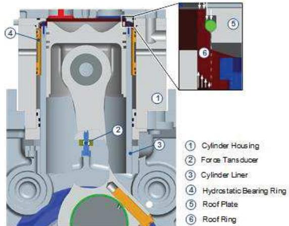
Figure 1 Floating-liner measurement system.
