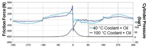
Figure 4 Motored crank-angle resolved friction forces w/ cylinder head.
