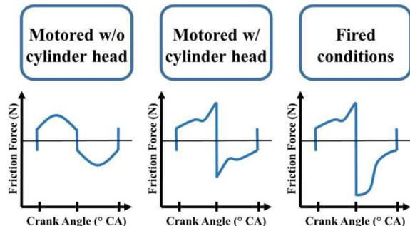
Figure 2 Operating modes for friction analysis.
