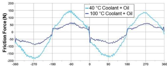
Figure 3 Motored crank-angle resolved friction forces w/o cylinder head.
