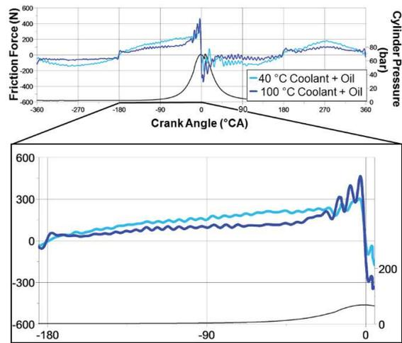
Figure 5 Fired crank-angle resolved friction forces.
