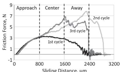
Figure 1 Friction force curve for JIS SUS316 at 8% RH in a ball-on-ball sliding test [4].
