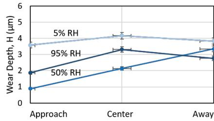
Figure 5 Wear depth against contact position (polished).
