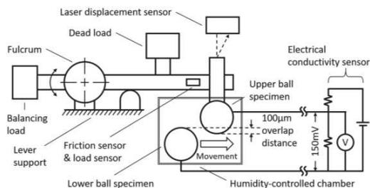
Figure 2 Schematic of a unidirectional ball-on-ball sliding tester [4].
