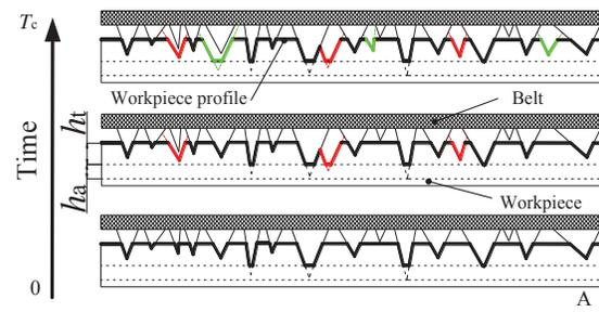
Figure1 The evolution of forming surface texture.
