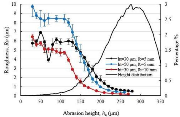
Figure 3 Roughness  $Ra$  vs. wear height  $h_a$ .
