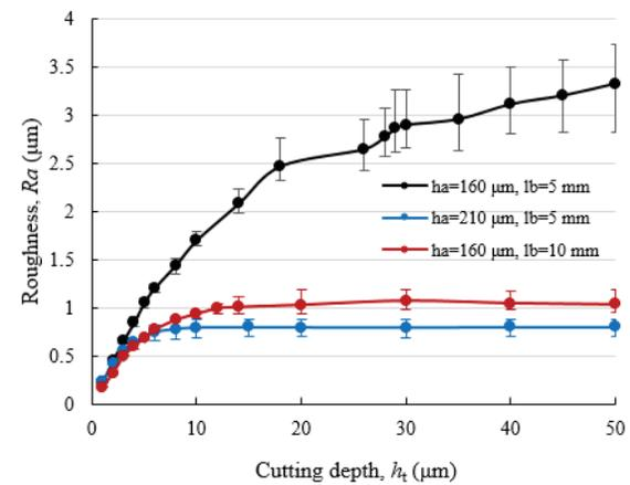
Figure 4 Roughness  $Ra$  vs. cutting depth  $h_t$ .
