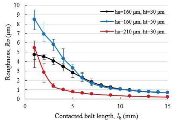
Figure 5 Roughness  $Ra$  vs. contacted belt length  $l_b$ .
