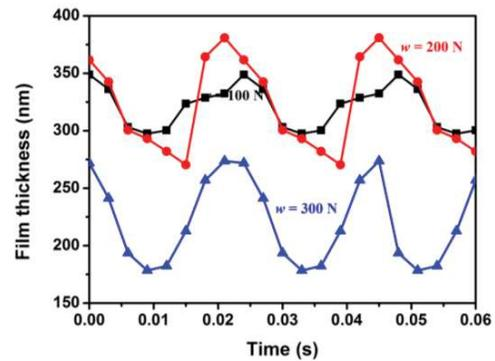
Figure 6 Variation of film thickness with time at different loads ( $u = 0.107 \text{ m/s}$ ,  $v = 242 \text{ mm}^2/\text{s}$ ).
