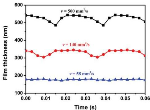
Figure 5 Variation of film thickness with time at different viscosities ( $w = 200 \text{ N}$ ,  $u = 0.107 \text{ m/s}$ ).
