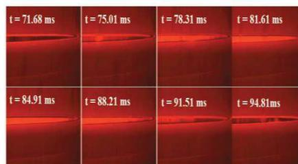
Figure 2 Variation of the oil film interference image in one cycle (corresponding to B in Figure 1) [1].
