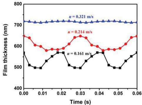
Figure 4 Variation of film thickness with time at different speeds ( $w = 200 \text{ N}$ ,  $v = 1000 \text{ mm}^2/\text{s}$ ).
