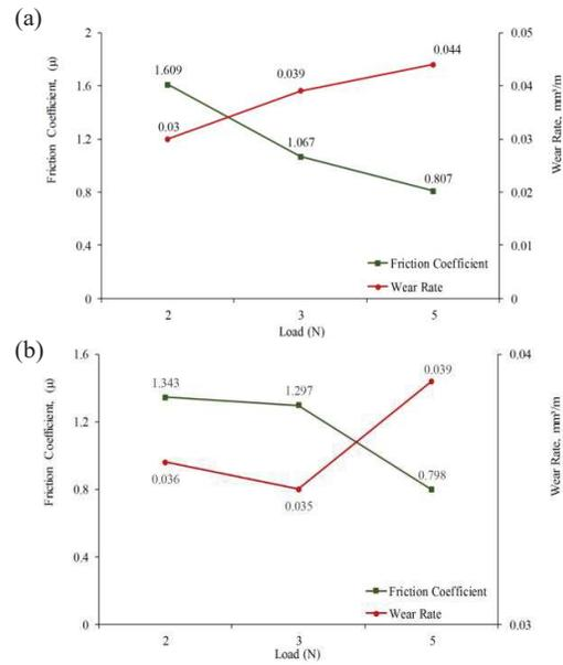
Figure 3 Friction coefficient and wear rate of (a) HPCS and (b) LPCS processes.
