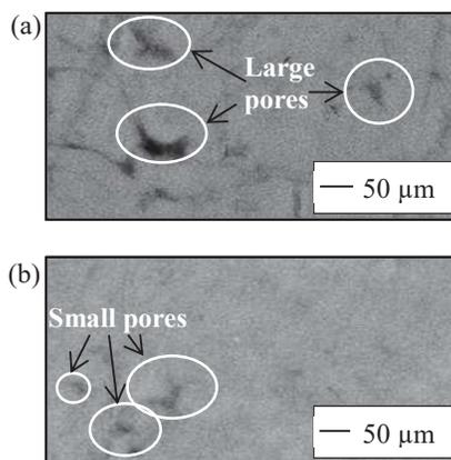
Figure 1 SEM images of Al coatings using (a) HPCS and (b) LPCS processes.
