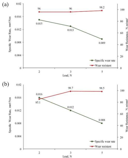
Figure 2 Specific wear rate and wear resistance of (a) HPCS and (b) LPCS processes.
