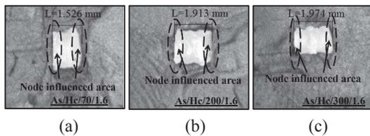
Figure 3 Strut effective length of lattice structure with layer thickness of (a) 70 μm, (b) 200 μm and (c) 300 μm.
