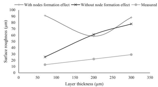
Figure 6 Layer thickness effect on surface roughness of lattice structure's struts.
