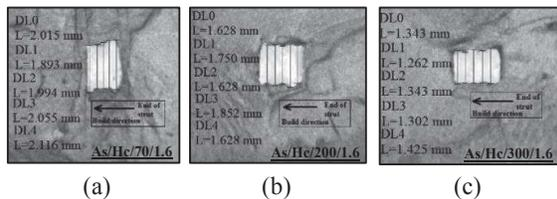
Figure 5 Single strut diameter of lattice structure with layer thickness (a) 70 μm, (b) 200 μm and (c) 300 μm.
