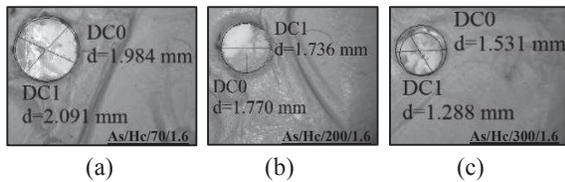
Figure 4 Minimum and maximum diameter cross section of lattice structure with layer thickness (a) 70 μm, (b) 200 μm and (c) 300 μm.
