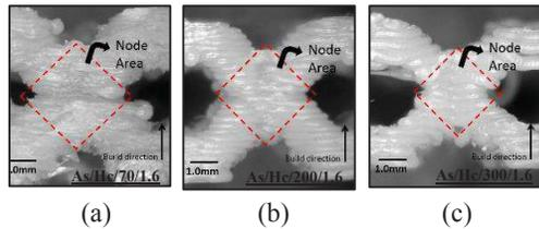
Figure 2 Node area in lattice structure with layer thickness of (a) 70 μm, (b) 200 μm and (c) 300 μm.
