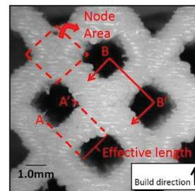
Figure 1 Details of node area, strut effective length and strut cross section.
