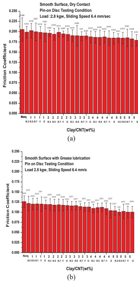
Figure 2 Pure sliding pin on disc testing on smooth surface. (a) Dry contact, (b) grease lubricated.
