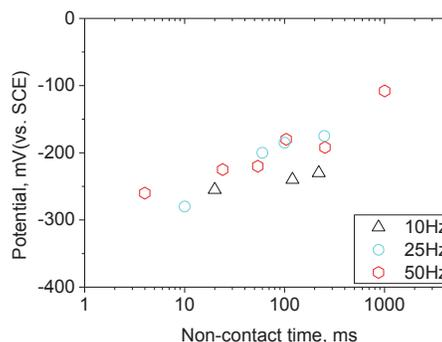
Figure 5 Average surface potentials of 304 stainless steels under impact fretting in Na<sub>2</sub>SO<sub>4</sub> solution (Temp. at 30°C, Impact load at 3N, Amp. at 50 $\mu$ m).
