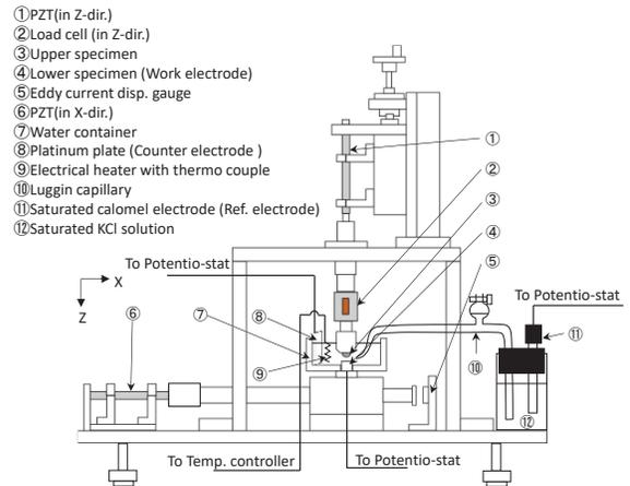
Figure 1 Schematic diagram of the impact fretting test rig.
