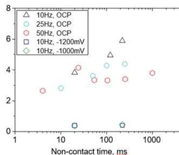
Figure 3 Relationships between the maximum wear depth and the non-contact time of 304 stainless steels against Al<sub>2</sub>O<sub>3</sub> ball in Na<sub>2</sub>SO<sub>4</sub> solution (Temp. at 30°C, Impact load at 3N, Amp. at 50 $\mu$ m).
