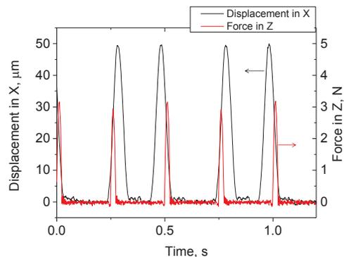
Figure 2 Measurement of displacement in X dir. and contact force in Z dir. (Impact load: 3N, Amp. in X dir.: 50 $\mu$ m, Frequency in X dir.: 10Hz, Interval time: 200ms).
