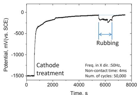
Figure 4 Surface potential of 304 stainless steel in impact fretting wear test (Temp. at 30°C, Impact load at 3N, Amp. at 50 $\mu$ m).
