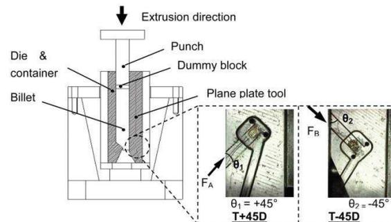
Figure 1 Plane strain extrusion apparatus and detection part of the frictional force.
