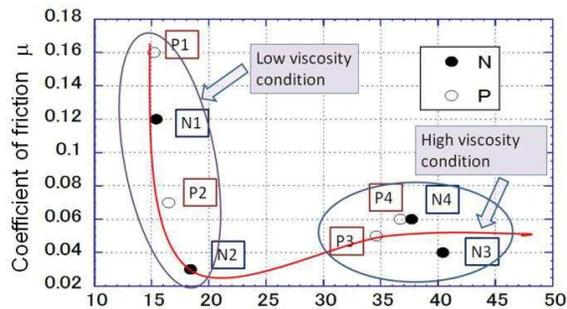
Figure 3 Coefficient of friction with regard to surface roughness parameter  $S$ .
