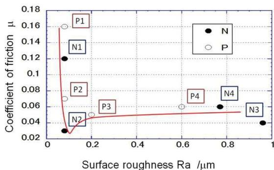
Figure 2 Coefficient of friction with regard to surface roughness parameter  $R_a$ .
