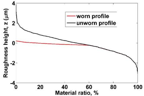
Figure 3 Bearing area curve (BAC) for unworn and worn profiles.
