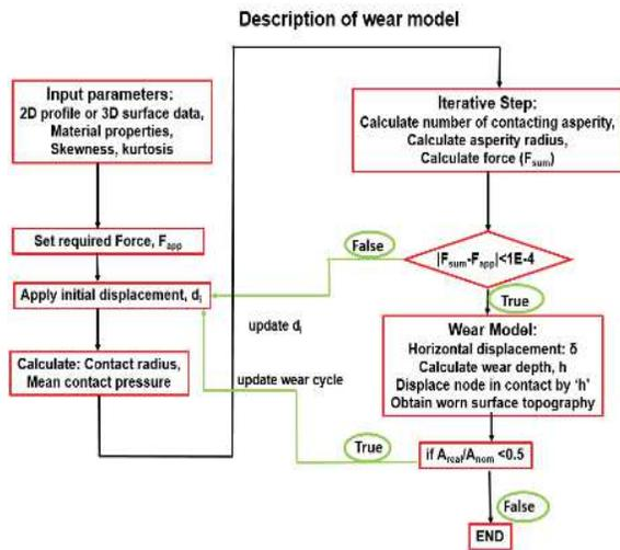
Figure 1 Flow diagram for wear simulation.
