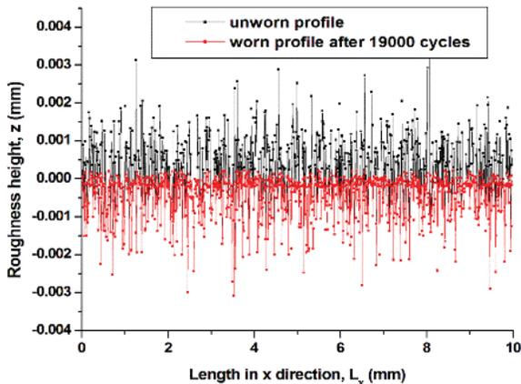
Figure 2 Unworn profile and worn profile after 19000 wear cycles.
