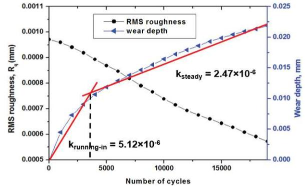
Figure 4 Change in RMS roughness and wear depth with number of cycles.
