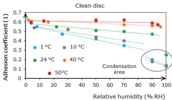
Figure 2 Influence of relative humidity and temperature on adhesion for clean disc.
