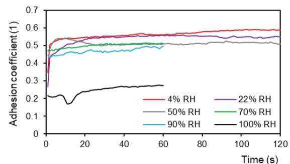
Figure 1 Effect of RH on adhesion for clean disc at air temperature 24  $^{\circ}\text{C}$ .
