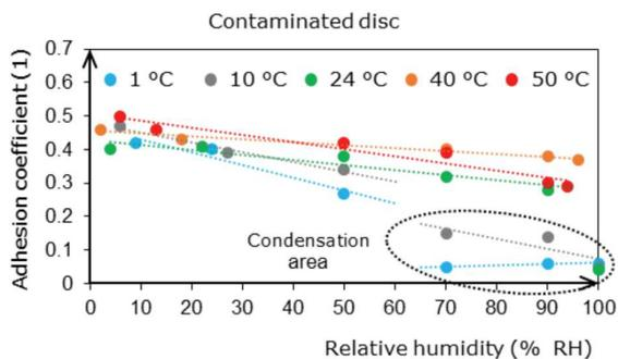
Figure 3 Influence of relative humidity and temperature on adhesion for contaminated disc.
