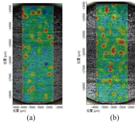
Figure 4 Raman mapping of carbon in pin surface; (a) Low humidity (0.7ppm), (b) High humidity (60ppm).
