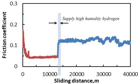
Figure 2 Friction coefficient with sliding distance.
