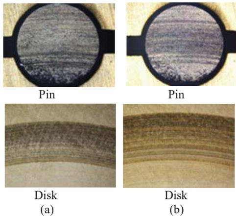
Figure 3 Pin and disk surface; (a) Low humidity (0.7ppm), (b) High humidity (60ppm).
