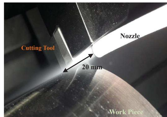
Figure 1 Position of the nozzle.
