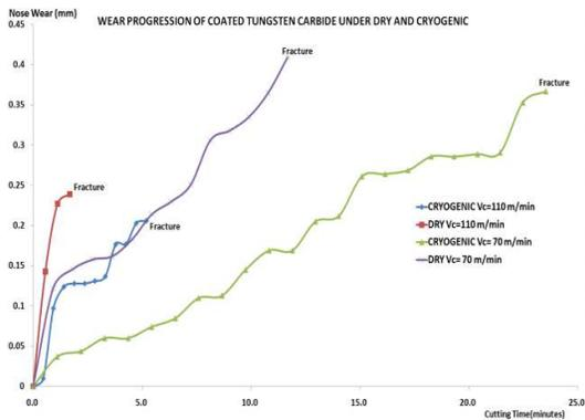
Figure 2 Wear progression under cryogenic and dry condition at  $V_c = 70$  and  $110$  m/min with constant  $f = 0.075$  mm/rev and  $a_p = 0.1$  mm.
