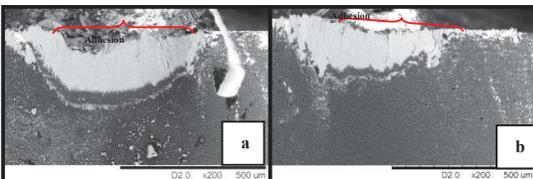
Figure 4 Wear mechanism at  $V_c = 110$  m/min for (a) dry and (b) cryogenic from nose view.
