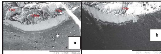
Figure 6 Wear mechanism at  $V_c = 110$  m/min for (a) dry and (b) cryogenic from tool edge view.
