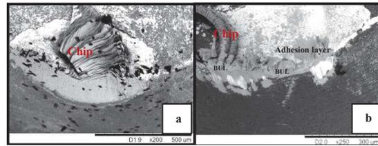
Figure 5 Wear mechanism at  $V_c = 70$  m/min for (a) dry and (b) cryogenic from tool edge view.
