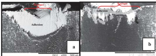
Figure 3 Wear mechanism at  $V_c = 70$  m/min for (a) dry and (b) cryogenic from nose view.
