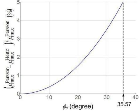
Figure 3 Ratio of the difference in the contact traction peak.
