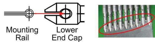
Figure 1 Conformal contact configuration of the SFR fuel rods.
