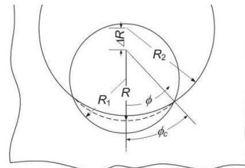
Figure 2 Geometrical model of a cylinder-hole contact.
