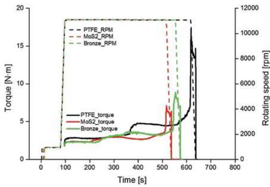
Figure 3 Torque changes with various composite solid lubricants.
