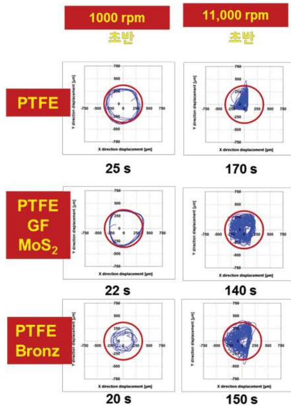
Figure 5 Cage center-of-mass orbits for cryogenic ball bearing with different solid lubricant.
