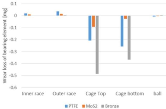
Figure 4 Wear loss of various composite.
