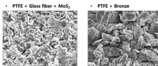
Figure 1 Microstructures of composite powders.
