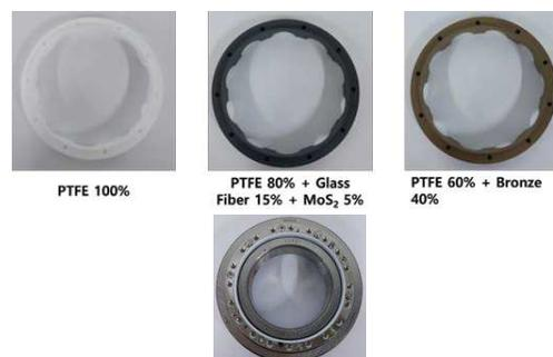
Figure 2 Composite cages and assembled ball bearing.
