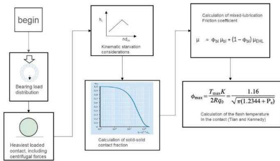
Figure 2 Flow chart depicting the model used to assess the risk of seizure in rolling bearings.
