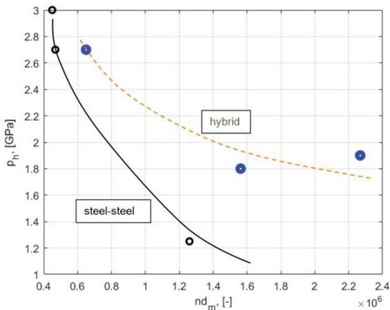
Figure 3 Maximum Hertzian pressure versus speed in the cases of experimental ball bearings with signs of raceway overheating. Superimposed sketched lines indicating the possible location of the onset of seizure failures for steel-steel and hybrid bearings.
