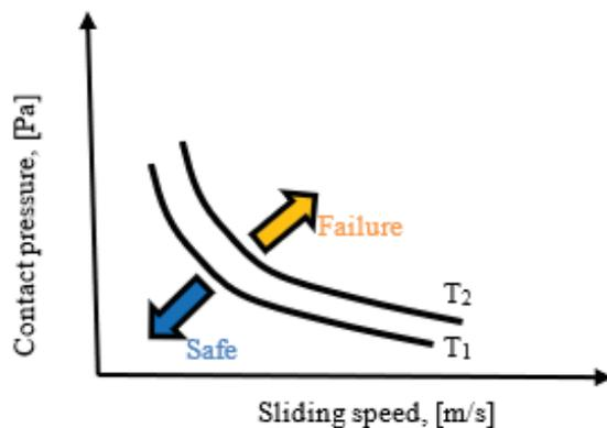
Figure 1 Schematics of a transition diagram of contact failure by seizure.
