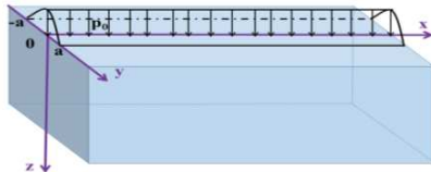
Figure 2 The model of finite-length elastic space.
