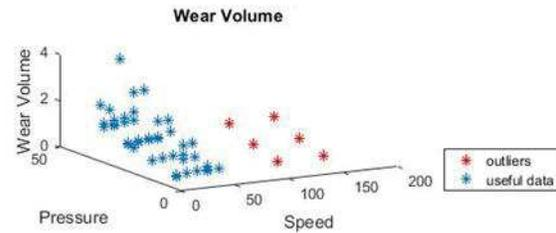
Figure 2 Wear volume experimental data with highlighted outliers.
