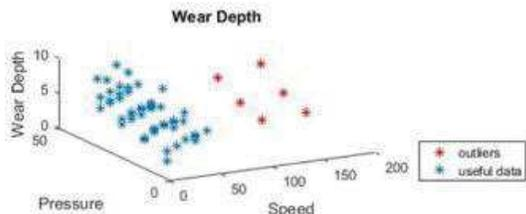
Figure 1 Wear depth experimental data with highlighted outliers.
