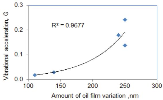
Figure 9 Relationship between oil film thickness variation and bearing vibration value.
