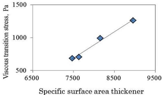
Figure 5 Relationship between specific surface area of thickener and viscous transition stress.
