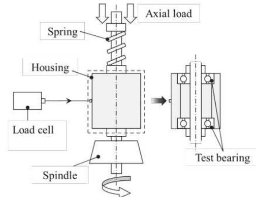
Figure 1 Bearing rotation torque measurement method.
