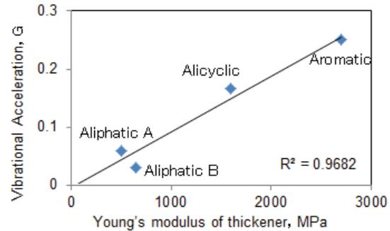
Figure 7 Relationship between Young's modulus of thickener and vibrational acceleration.
