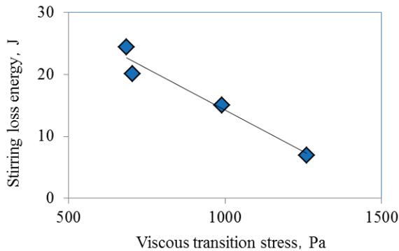
Figure 4 Relationship between viscous transition stress and stirring loss energy.
