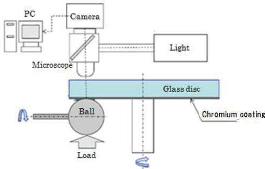
Figure 3 Oil film thickness measuring equipment.
