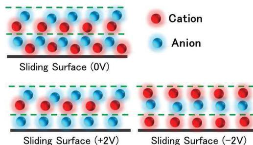
Figure 3 the model diagram of ionic liquids against surface electric potential.
