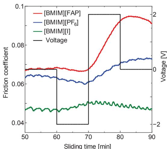
Figure 2 Friction behaviour of each ionic liquid.
