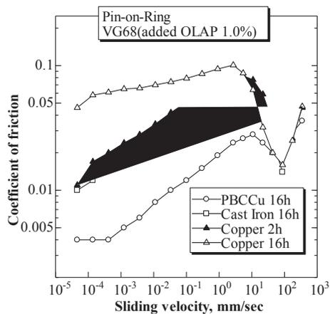
Figure 2 Boundary friction properties of these experimental results.
