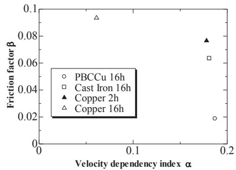
Figure 3 The relationship between velocity dependence and friction factor.
