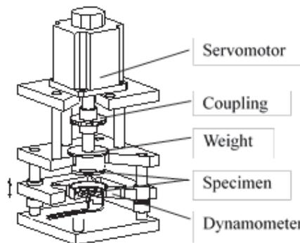
Figure 1 Schematic of experimental apparatus.
