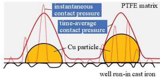
Figure 4 Possible contacting pressure distribution after running-in.
