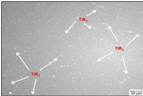
Figure 3 Microstructure of Al-15wt.% $TiB_2$  MMC.
