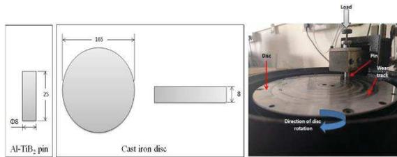
Figure 2 Pin on disc setup.
