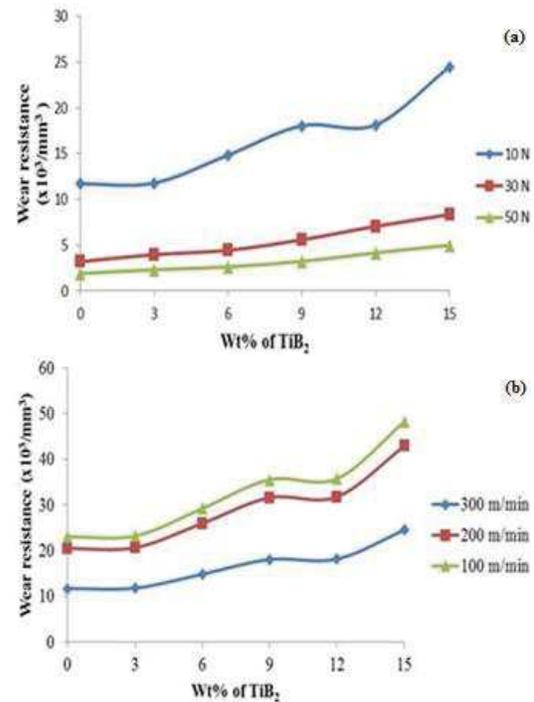
Figure 4 Wear resistance as a function of weight percentages for varying (a) load and (b) speed.
