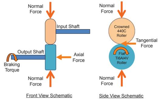
Figure 2 Schematic of the test rollers and forces.
