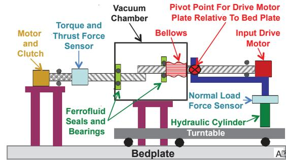
Figure 1 Schematic of the VRR, side view.
