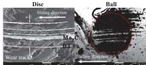
Figure 4 SEM image of Si-DLC and SUJ2 ball surface after friction test in PAO with 0.1 wt.% of Mo<sub>2</sub>C.
