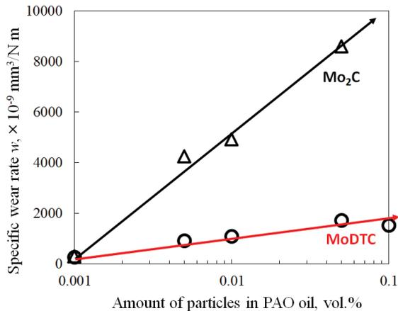
Figure 2 Specific wear rate of Si-DLC against SUJ2 ball in PAO with MoDTC or Mo<sub>2</sub>C.
