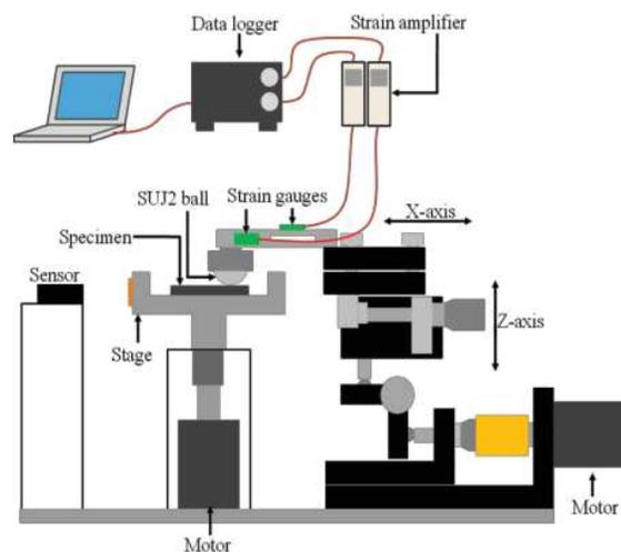
Figure 1 The schematic image of Ball-on-Disc friction tester.
