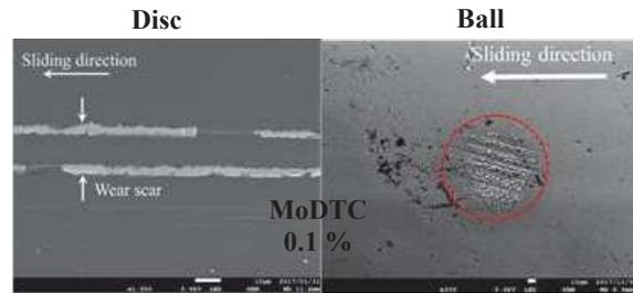
Figure 3 SEM image of Si-DLC and SUJ2 ball surface after friction test in PAO with 0.1 wt.% of MoDTC.
