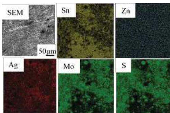
Figure 2 SEM/EDX image of Ag-MoS<sub>2</sub> containing coating film.
