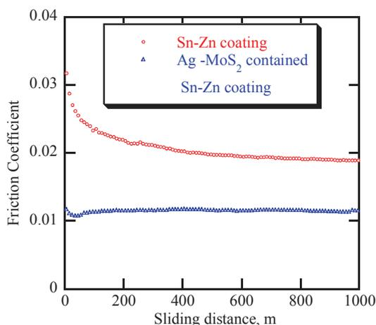
Figure 3 Friction coefficient of coating surface as a function of sliding distance.
