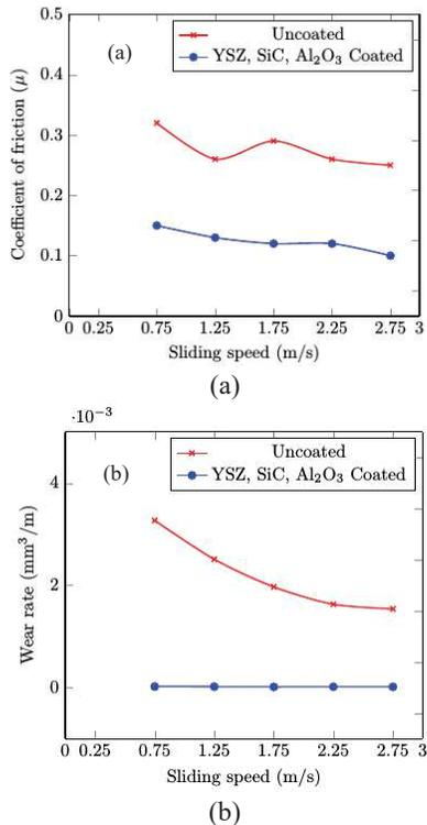
Figure 1 Tribological characteristics (a) Wear rate against sliding speed and (b) coefficient of friction against sliding speed.
