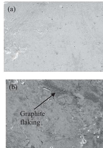
Figure 4 (a) Surface profile at 66 m/min and (b) surface profile at 99 m/min.
