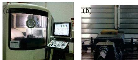
Figure 2 (a) DECKEL MAHO DMU 60 milling machine and (b) machining setup.
