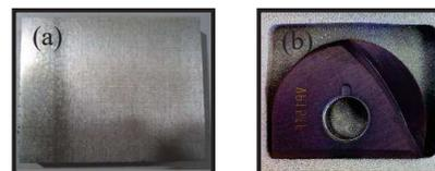
Figure 1 (a) FC300 gray cast iron and (b) SRFT 30 VP15TF TiAlN coated ball end mill.
