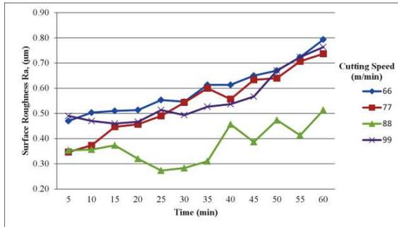
Figure 3 Surface roughness against cutting time at a feed rate 5000 mm/min.
