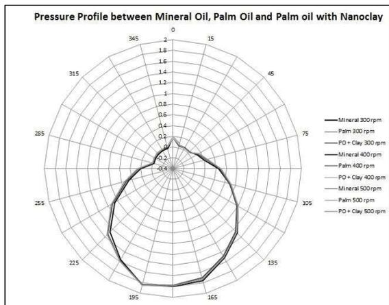
Figure 2 Pressure profiles of mineral oil, palm oil in and palm oil with Nanoclay at 10 kN for different speeds.
