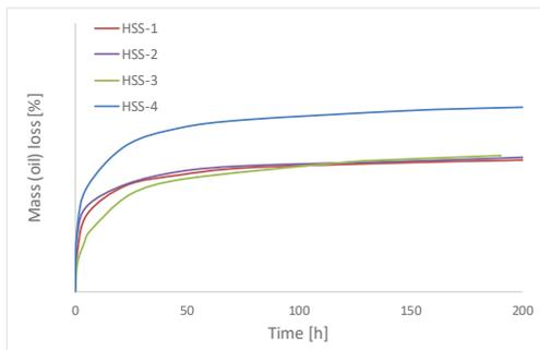
Figure 3 Dynamic oil bleeding (centrifugal force).
