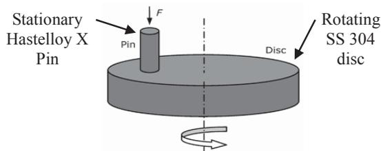
Figure 1 Schematic diagram of pin and disc.
