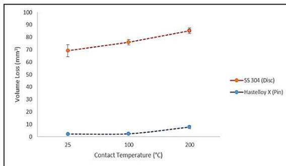
Figure 2 Volume losses against contact temperature of SS304-Hastelloy X tribo-pair.
