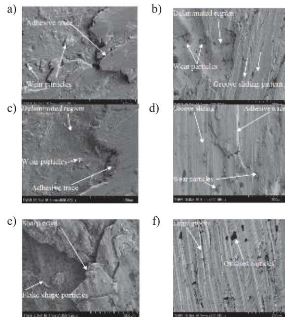
Figure 4 Morphologies of worn surfaces for SS304-Hastelloy X tribo-pair at 25°C pin (a), 25 °C pin (b), 100 °C pin (c), 100 °C disc (d), 200 °C pin (e) and 200 °C disc (f).
