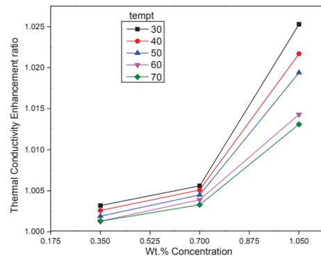
Figure 1 thermal conductivity enhancement ratio for all concentrations under varying temperature.
