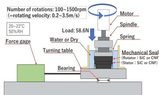
Figure 1 Schematic drawing of experimental apparatus of friction test [5].
