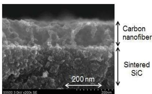
Figure 2 Cross section of CNF film on sintered SiC substrate observed by SEM [5].
