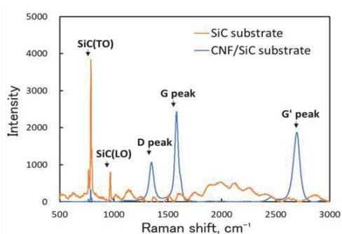
Figure 3 Raman spectra of SiC substrate and CNF film on sintered SiC substrate [5].
