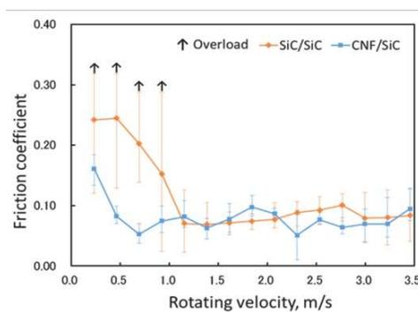
Figure 4 Friction coefficient under water condition as a function of rotating velocity [5].
