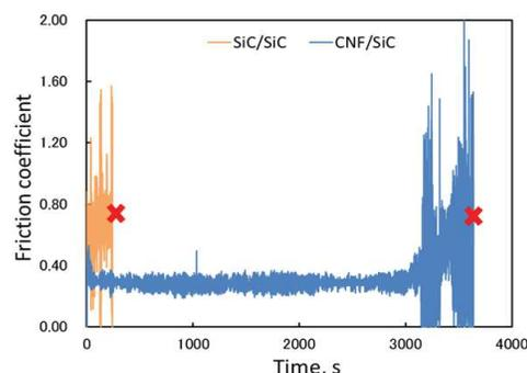
Figure 5 Friction coefficient under dry condition as a function of experiment time [5].
