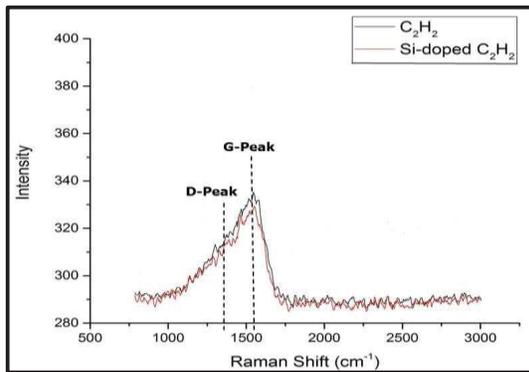
Figure 1 Raman graph of non-doped and Si-doped DLC sample.
