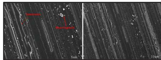
Figure 5 SEM images of Si-doped DLC sample.
