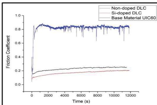
Figure 2 Friction coefficient of untreated, non-doped and Si-doped DLC sample.
