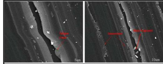
Figure 4 SEM images of non-doped DLC sample.
