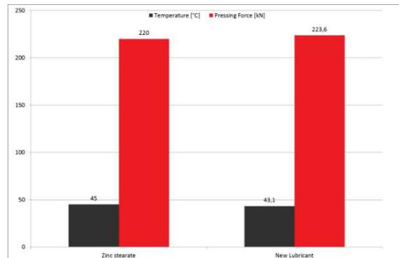
Figure 5 Temperatures and pressing forces at the field test.
