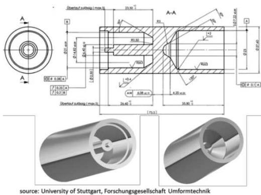
Figure 3 Drawing of the field test part.
