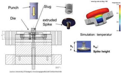
Figure 2 Design of the spike test tool.
