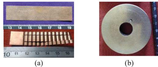
Figure 7 (a) Top and bump foil. (b) Assembly of foils with bearing base.
