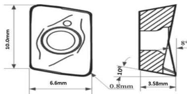
Figure 1 Cutting tool geometry for DNMA432.
