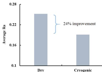
Figure 2 Comparison of a for dry and cryogenic conditions or for test 4.
