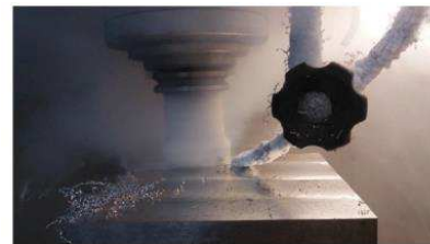
Figure 1 Delivery of liquid nitrogen during the high-speed milling process.
