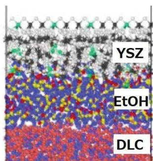
Figure 1 Molecular dynamics simulation of the friction of confined system between YSZ and DLC, and ethanol molecules. Chemical reaction is treated by Reax Force Field.
