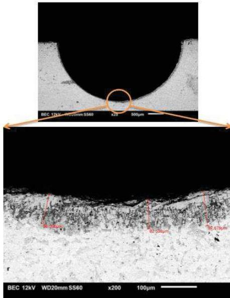
Figure 2 SEM cross-section image of C-shape groove at 1123 K for 6 hours.
