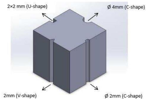
Figure 1 Schematic of grooved surfaces specimen.
