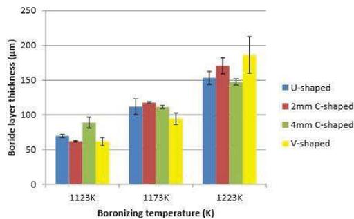
Figure 3 Boride layer thickness for different grooved surfaces at 6 hours duration.
