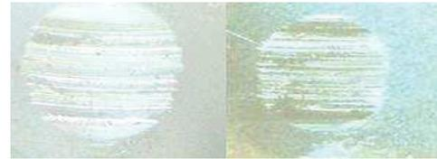
Figure 4 Wear scar diameters.
