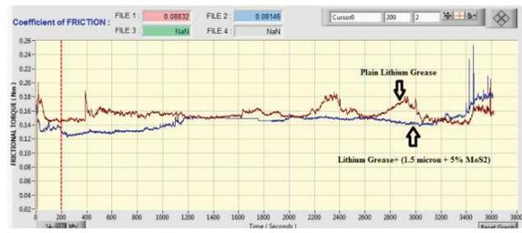
Figure 3 Comparison of frictional torque.
