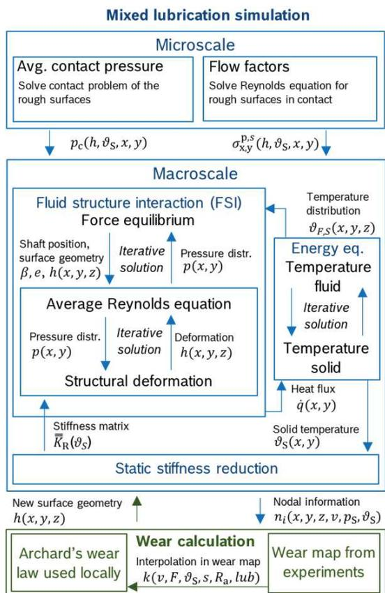
Figure 2 Basic simulation framework of the macroscale mixed lubrication simulation with a wear calculation loop.
