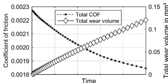
Figure 5 Wear and friction progress of 45 mixed lubrication simulations.
