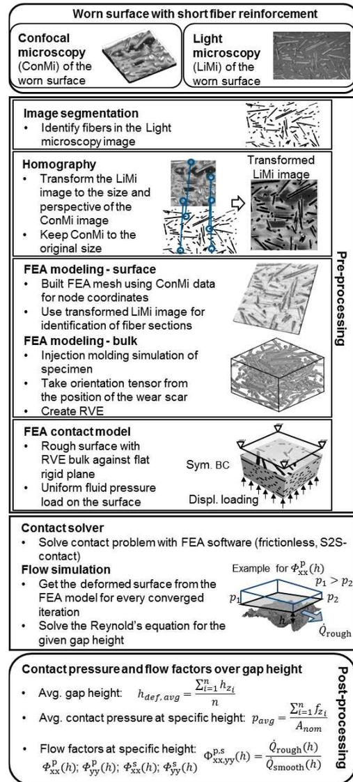
Figure 1 Simulation framework for calculating average contact pressure and flow factors of rough short fiber reinforced polymer surfaces [5].
