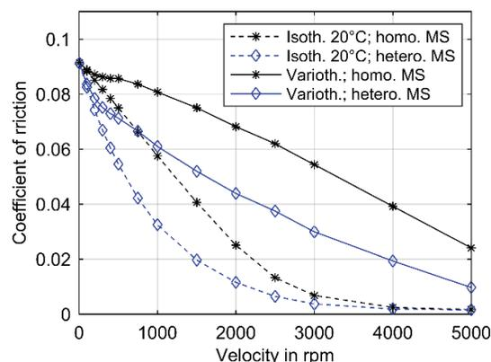
Figure 4 Stribeck curves - Comparison of isothermal and variothermal calculation with homogeneous resp. heterogeneous microstructure (MS) for ideal cylindrical shapes.
