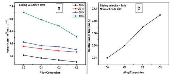
Figure 5 (a) variation of wear rate with composition, (b) variation of coefficient of friction with composition.
