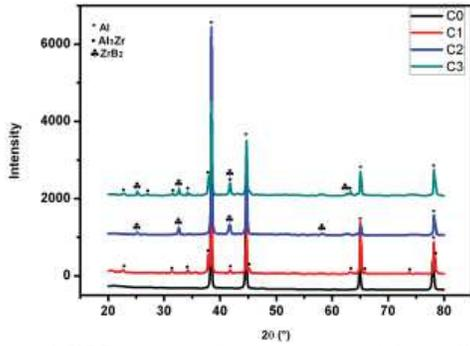
Figure 1 XRD pattern of composites with base alloy.
