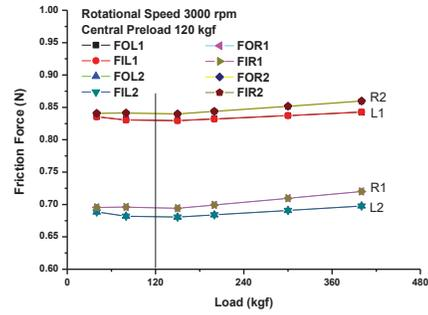
Figure 4 Friction forces VS axial load.
