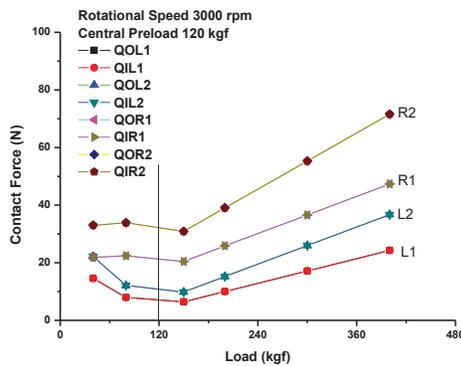
Figure 3 Contact forces VS axial load.
