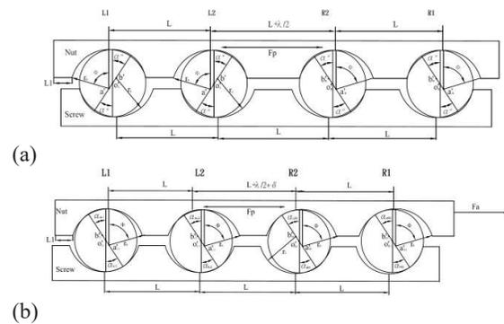
Figure 1 Sketch of four-cycle ball-screw, (a) without external load, (b) with external load.
